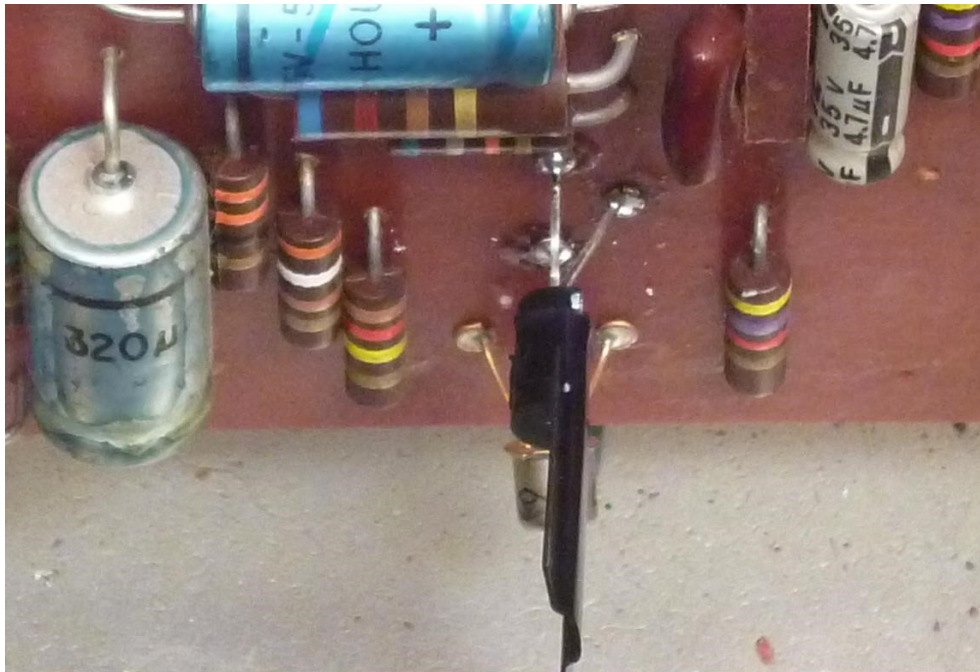
Figure 2-New transistor with heatsink installed on PCB
